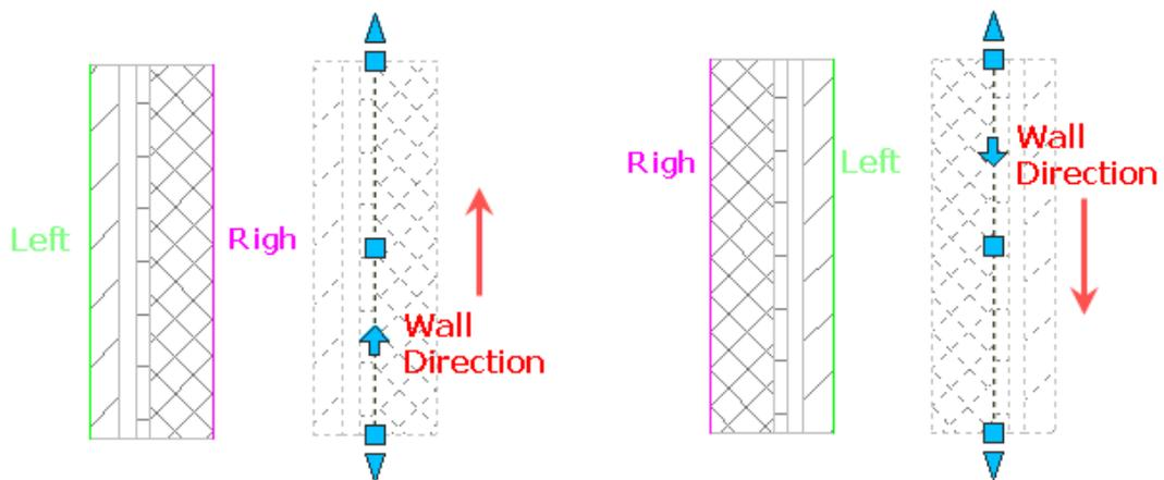
Association of composite wall left or right position with wall direction
