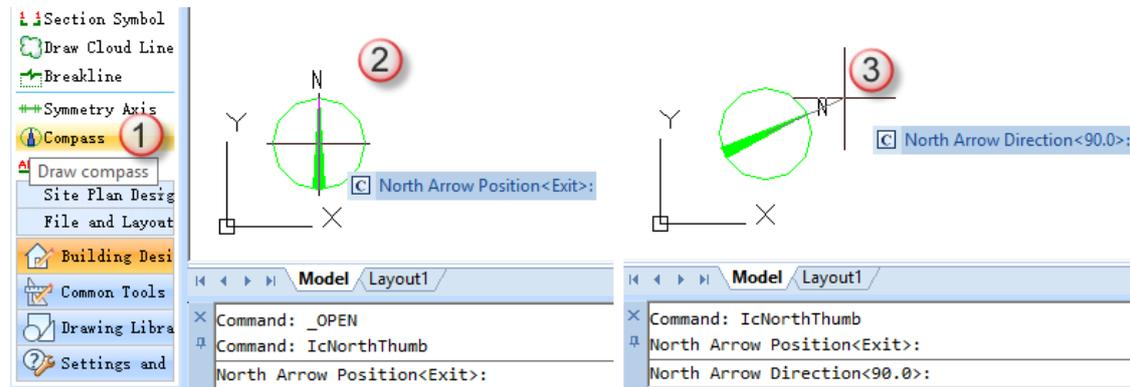
Operation Guide for Drawing Compass
