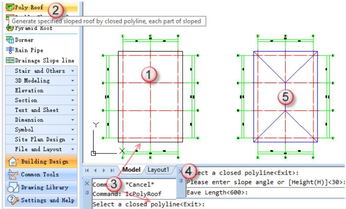
Operation Guide for Drawing Roof
